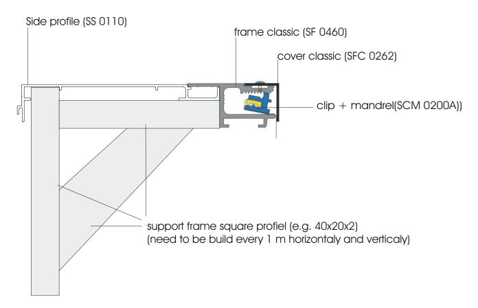
The fabric is tensioned with the help of the clips and the mandrels in the frame. You should begin with hanging in the fabric in the top of the box, afterwards the sides are tensioned. When the fabric is without any wrinkles the bottom edge is tensioned.
